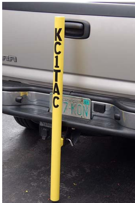
This is a receiver hitch antenna mount that Greg W1VFB and Don KB1LXH designed and had built for the Hurricane Awareness Tour. The right hand picture is the mount with a 23 foot mast and a Cushcraft R-5 multi-band antenna that Bruce N11X loaned to the Group for the event.
