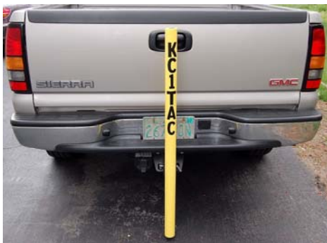
This is a receiver hitch antenna mount that Greg W1VFB and Don KB1LXH designed and had built for the Hurricane Awareness Tour. The right hand picture is the mount with a 23 foot mast and a Cushcraft R-5 multi-band antenna that Bruce N11X loaned to the Group for the event.
