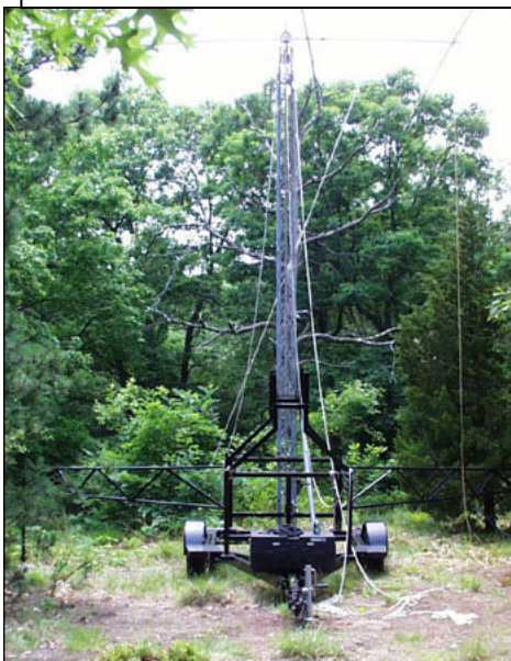
The crank-up tower designed and built by members of the SMHARC.
